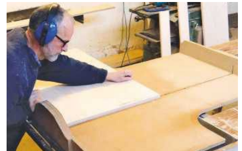
▲ Pic.4 Richard has built a cradle with which to cross-cut sheet material as accurately as he rips it. It runs in the guide slots of the table saw. It would not work if the saw blade were guarded. The cradle provides firm holding for the sheet. Keeping the workpiece under tight control is of prime consideration in safe woodworking
